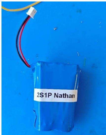
Fig.16 2S1p Li-ion battery pack finalized
